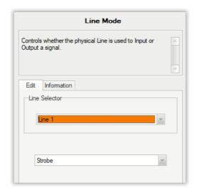
In such situation selected parameter is connected with one of categories (slots) described by selector. In the example on the above image, parameter is determining whether the physical Line is used to Input or Output a signal. This device has two lines and both have its own separate values to choose from. Selector will pick which line we want to edit and bottommost editor will change it purpose. This means that there are actually two different *Line Modes* parameters in device.
